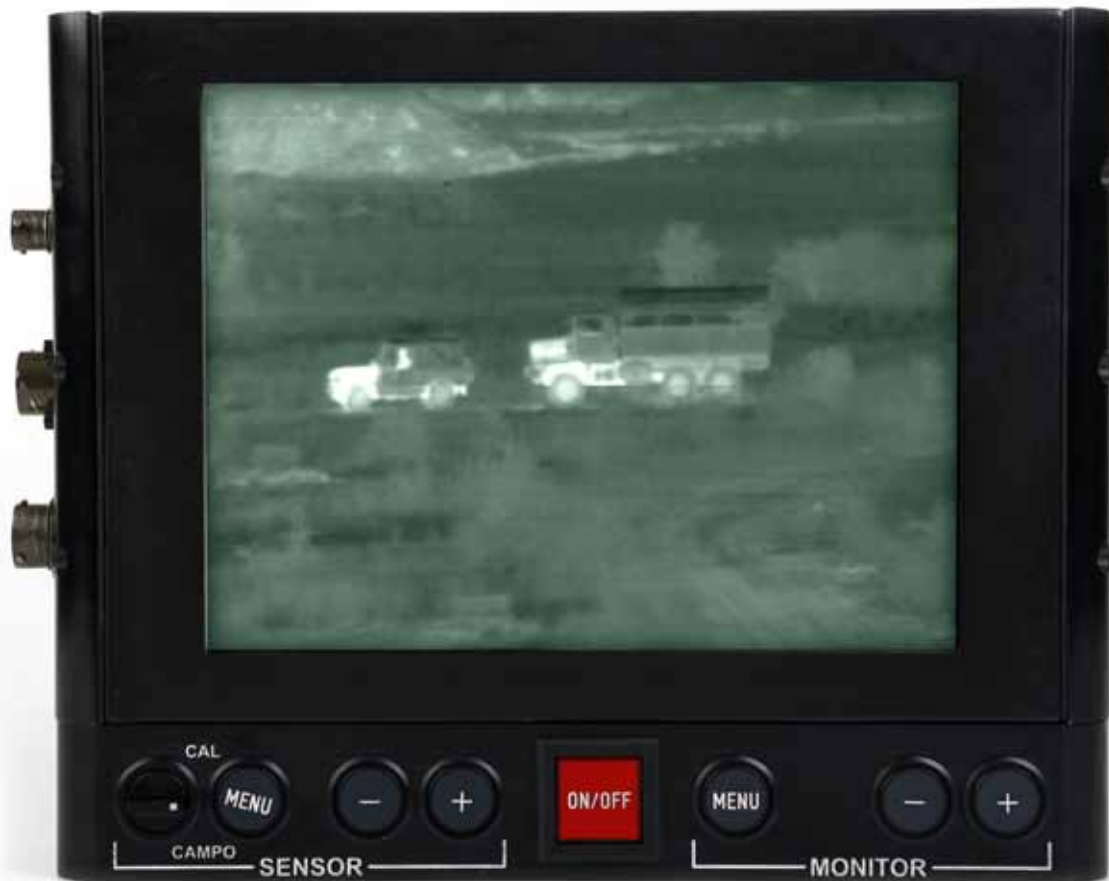
Integrated monitor and sensor control
