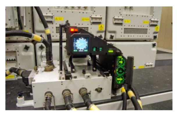
SAMe is a Standard Automatic Test System for Intermediate and Depot Level maintenance of modern avionics and electronic systems
