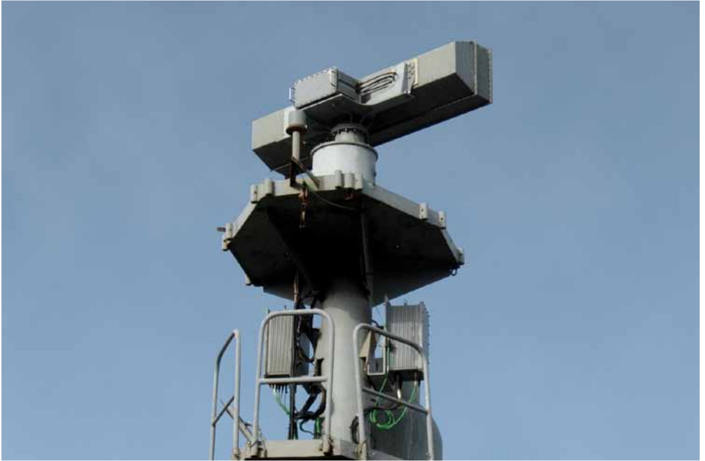
ARIES-SAAS installed on a ship
