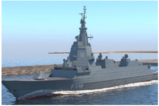
F110 (2020-2027) Integrated frigate mast
