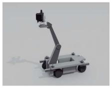
Portable 3D image acquisition system with different capabilities to produce a 3D model in real time:
