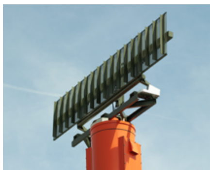
Secondary Surveillance Radar / IFF
