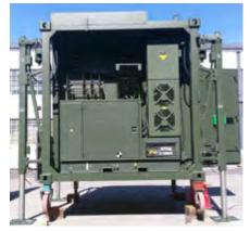
This unit provides a local radar operator interface with the radar sensor and displays the air picture as seen by the radar. This unit also provides the operator with means to control and monitor the radar and IFF operation and includes the interface for the possible integration and exchange of information with the Air Defence C2 Center via data link with the support of radio and/or optic fiber.
