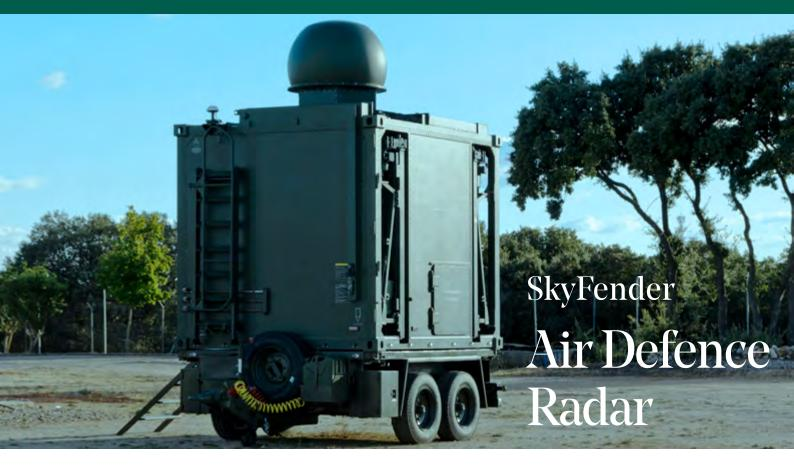
SkyFender ADR is an X-band pulse-doppler radar designed to provide real-time air surveillance to detect multiple target types flying at low and very low altitudes, even in low visibility and harsh weather conditions
