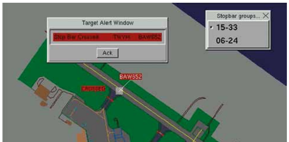
An aircraft after crossing the stop bar with the alarm function on
